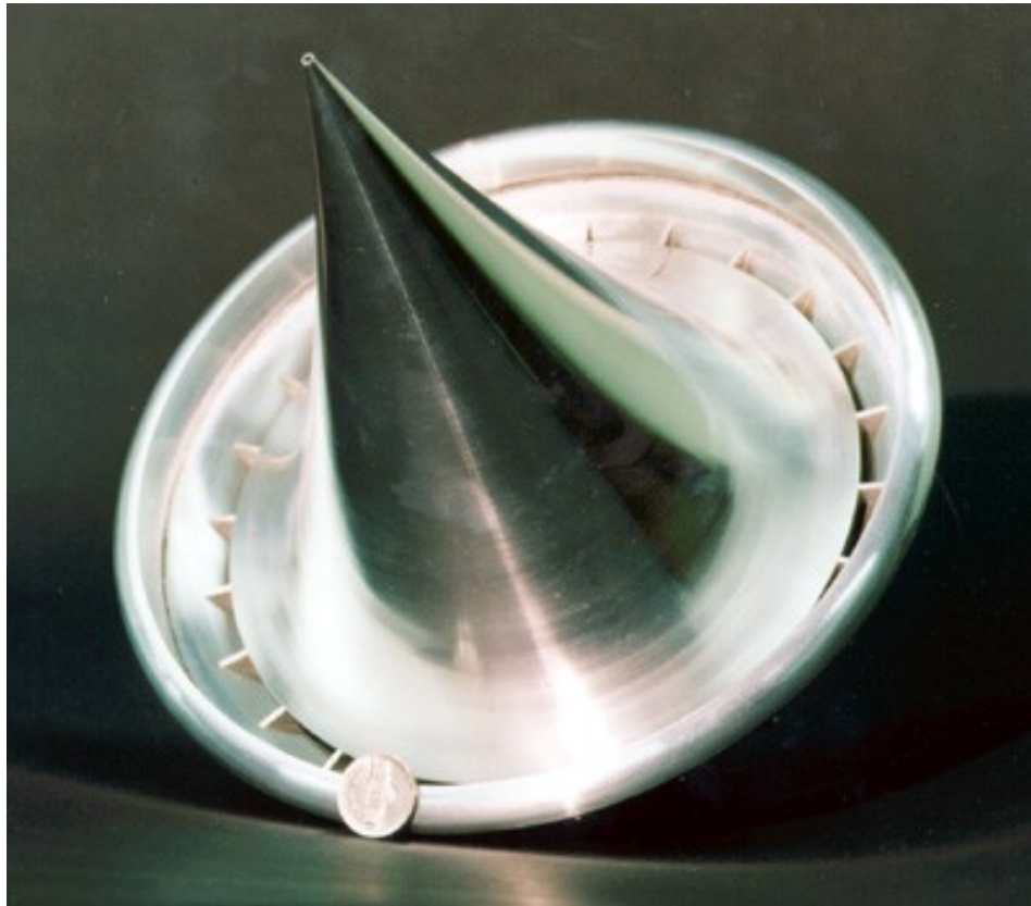
LightCraft Model Object (Rear view of laser light entry tip)
