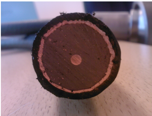
Figure 2.13: A cross section of the coaxial cable. Both the inner and the outer conductor is visible, along with the dielectric filling the void between the two. A rubber shield sits on the outside to protect the cable and the surrounding.
