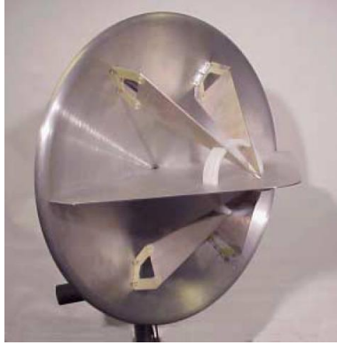
Figure 3.10: One IRA having a ground plane. [13]
